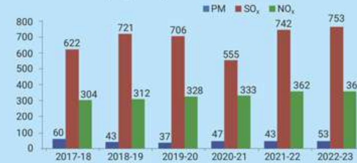
WBDCL - Bakreswar Thermal Power Station Emission Data (mg/Nm 3 )
