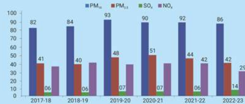
WBPDC - Bakreswar Thermal Power Station Ambient Air Data ( \mu\text{g}/\text{m}^3 )
